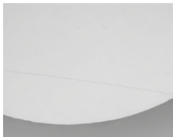
Scratched mirror-finished surface
