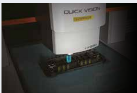
Example of measuring an engine control unit
