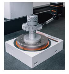
Software: MCOSMOS Probe System: PH10MQ, SP25 Work piece: Mitutoyo Demo piece
