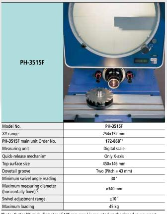
Photo: Cutter (Outside diameter of 175 mm max.) is mounted on the tipped-saw support fixture (172-001).
