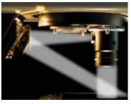
The Surface illumination comprises vertical illumination, which goes through the projection lens, and oblique illumination, with changeable angle of illumination emitter, as standard. It is effective in three-dimensional observation with enhanced color reproducibility.
