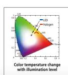
Color temperature varies significantly with the level of halogen illumination but not so much with LED illumination, so the appearance of the image varies a lot less as the LED level is adjusted. Also, the projected image under LED illumination is sharper and easier on the operator's eyes, which contributes to a reduction in fatigue and therefore more efficient inspection and measurement.
