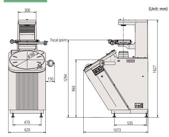
Note: To mount the counter (KA-212) and counter stand, approximately 300 mm space is required on the right-hand side of the main unit.
