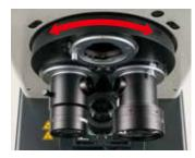
The turret of the PJ-H30 Series uses low-friction bearings that enable smooth and rapid rotary motion for changing magnification by bringing different projection lenses into the light path. The turret body uses bayonet mounts to aid quick attachment and detachment of lenses.
