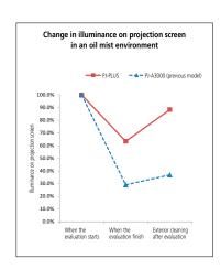
Adoption of the LED illumination source has obviated the need for installing a cooling fan into the main unit of the measuring instrument, and has drastically decreased the entry of oil mist, dust, etc. via the cooling fan into the instrument body.
