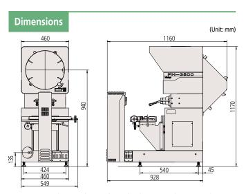
Note: To mount the optional counter (KA-212) and counter stand, approximately 300 mm space is required on the right-hand side of the main unit.
