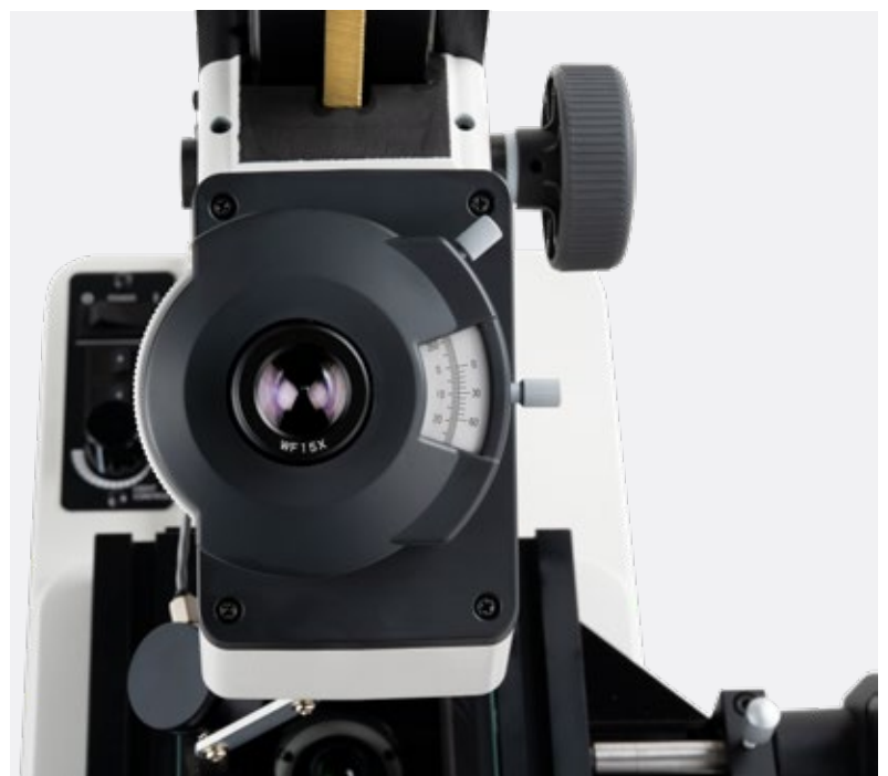
A vernier scale mounted outside the eyepiece enables simple angle measurement.
