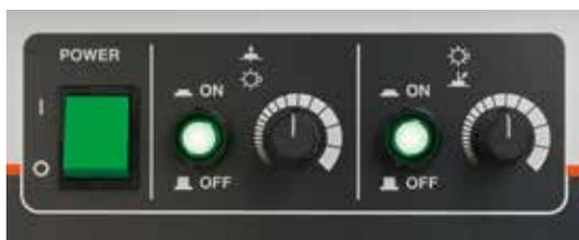
Stepless illumination adjustment has been adopted so as to provide moderate illuminance according to the surface texture and color of the workpiece. Illumination strength ranges from weak to strong and this method is also effective in extending the halogen lamp life, which is enhanced by using a soft start feature to limit inrush current.
