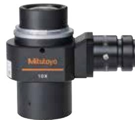
The projection lens is equipped with a C mount, therefore a compatible digital camera can be attached. Retrofit is possible Profile Projector (PJ-H). A workpiece can be observed on the large-size projection screen, and simultaneously the color image can be saved on the camera and observed on the monitor.
