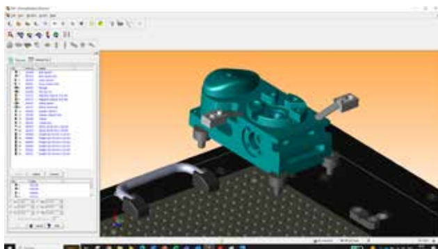
Applied of support points and clamps
